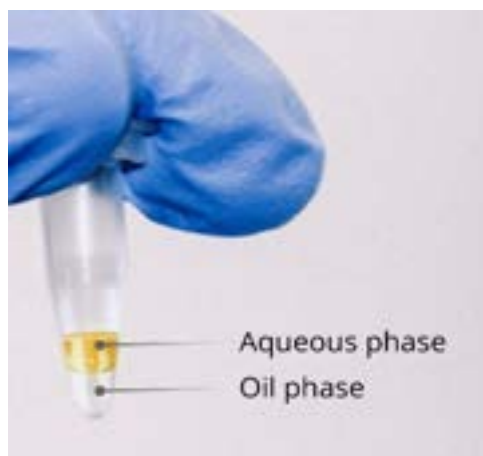
Figure 4.2. Break the droplets with Droplet break solution ● and Droplet break color ●. Keep the, colored aqueous phase.
