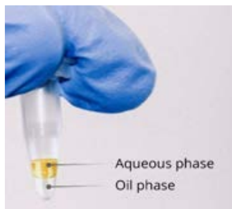
Figure 3.3 Break the droplets with Droplet break solution ● and Droplet break color ●. Keep the, colored aqueous phase.
