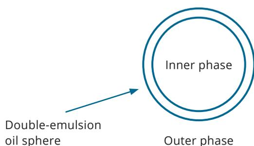
**Figure 1.** Xdrop double-emulsion droplet structure. They are composed of an oil sphere filled and surrounded by aqueous solutions (referred to as a water-in-oil-in-water system). The oil contains no components of animal origin, making the droplets suitable for animal cell analyses
