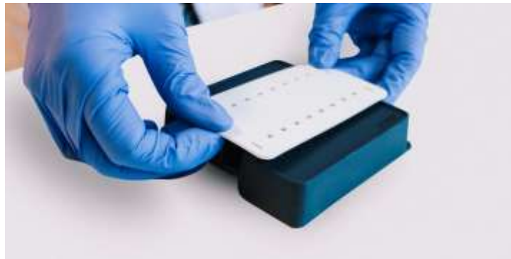
Fig. 5.6. Attach the white rubber gasket to T-hooks of the dMDA cartridge.
