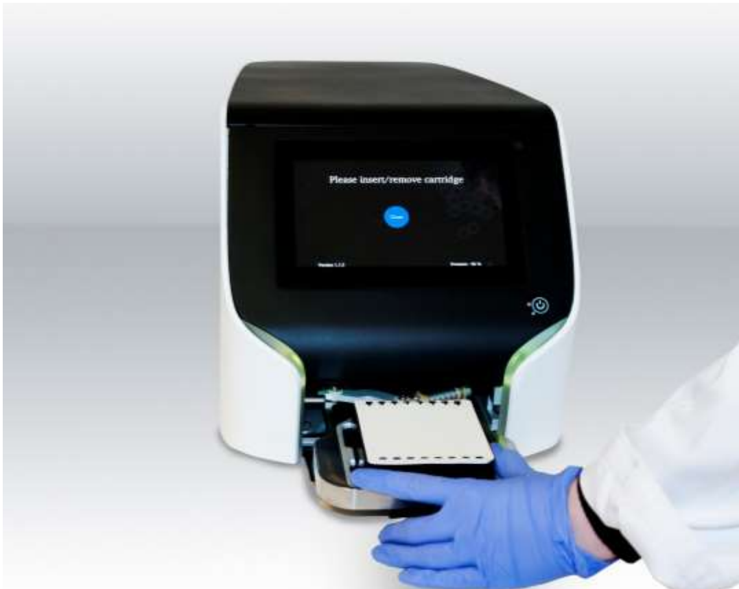
Fig. 3.5. The Xdrop instrument with a correctly inserted dPCR cartridge. Be very careful to position the cartridge correctly to avoid damaging the instrument or cartridge.
